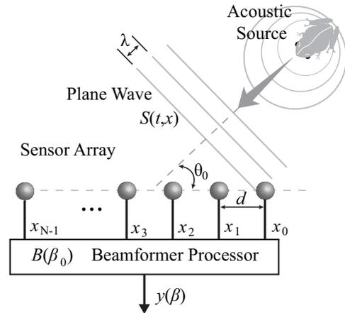
Fig. 5. Basic Beamforming Operation
